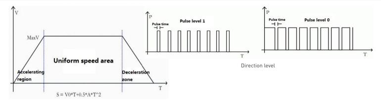
When the direction level of 1, the shaft is running, the Output is high level, Anti-run is low level. When the direction level of 0, the shaft is running, the Output is low level, Anti-run is high level.
