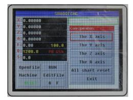
X-axis uniaxial cleared Y-axis uniaxial cleared Z-axis uniaxial cleared A shaft uniaxial cleared All axes cleared Exit Panel shortcuts ¤ «Manual and Joq»
