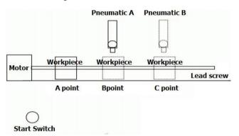
A position of the origin point, B point 500MM, C point 1000MM
