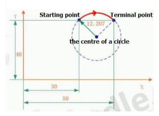
X, Y, Z Terminal point coordinates, F processing speed
