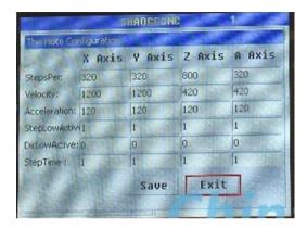
Acceleration: Maximum acceleration of the motor can run, this value is too small will be more seriously affected micro segment corner speed.
